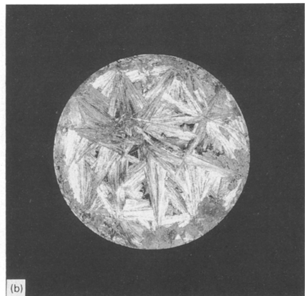
Figure 10 Macrographs of the top surfaces of alloys S2 (a) and S3 (b) made from commercially pure materials. The silicon content varied from 3.57 (a) to 7.1 wt % (b).
