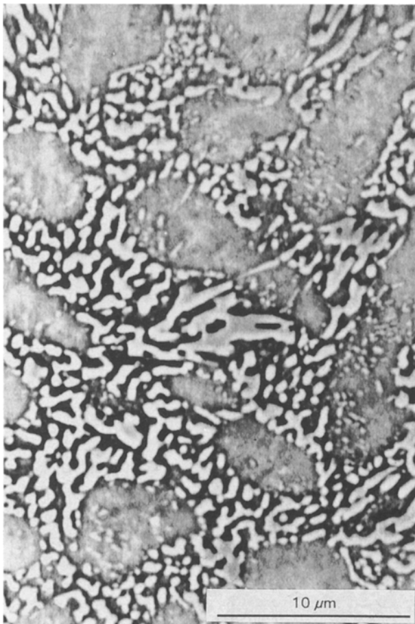
Figure 4 Typical area of sample in undercooled hypo-eutectic alloy similar to that of Fig. 3 subjected to EBSD.
