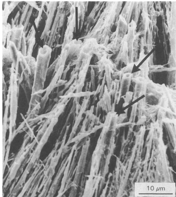
Figure 8 SEM micrograph of eutectic carbides near end of cell tip showing coarser carbides (arrows) around the periphery of the tip. Note holes in carbides from dissolution of matrix core by deep etching.
